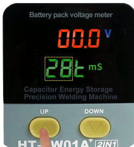
4. Set energy grade— Press the "▲" or "▼" button to increase or decrease energy grade.
