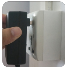
② Plug the adapter into an AC 100-240 volt wall socket to charge the machine.
