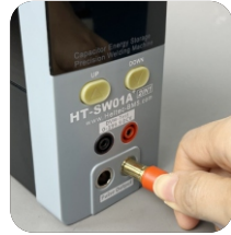
③ Insert the mobile welding pen and make sure the connection is solid.
