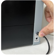
① Plug the power output plug into SW01A+ spot welder power connection port.
