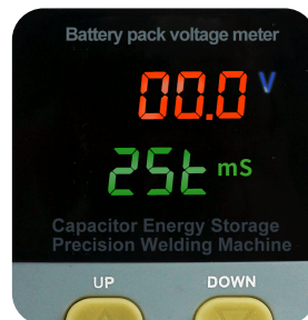
3. When the voltage is between 5.2 and 5.8V, the machine will display 25ms, that is ready for use.
