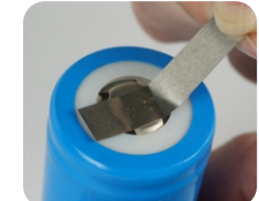
3. Check the spots' reliability. Finish spot welding.
