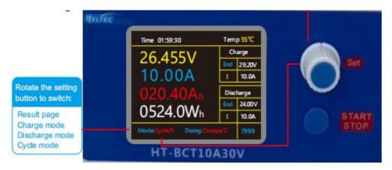
3. After waiting for the test to end, the result page will automatically pop up (press any button to stop the alarm sound) and record it manually. Test the results, and then test the next battery.
