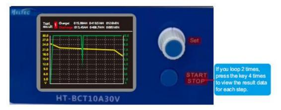
Test results: 1 indicates the first cycle, the AH/WH/min of charge and discharge respectively. Press the start / stop button further to show the results and curve of each step in turn.
