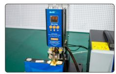
Press the foot switch and the pneumatic welding head will press down to start welding.
