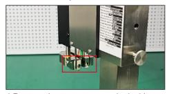
4.Remove the rear screws on both sides of the welding head
