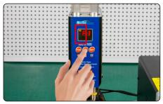
8.Press the "CAL" button again, the CAL red light goes out, and the simulated spot welding is exited.
