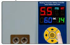
Adjust the spot welding machine output power according to the thickness and material of the workpiece to be welded.
