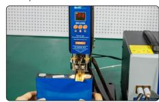
Confirm the pneumatic welding head pressure, speed and welding position based on the simulated spot welding.
