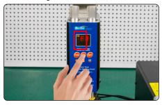
Press the "CAL" button, the red CAL light flashes, and step on the foot switch to simulate spot welding.
